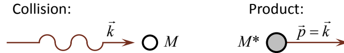
Figure A-2: Photoelectric absorption of a photon by a system with initial mass M (shown in the lab frame). The photon is destroyed by the interaction, and the mass of the target system is increased by the collision to the new value M^* > M . Conservation of momentum requires that the product M^* recoil with the incoming photon's momentum, requiring some of the incoming photon's energy.
