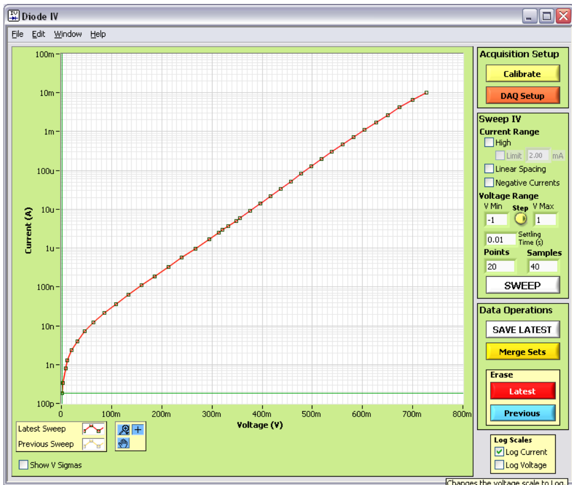
Figure 4: Diode IV Application Main Window. The displayed IV curve data is for a room-temperature silicon diode.
