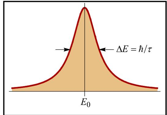
**Figure 2: Lorentzian distribution of the energies of an excited state with nominal energy  $E_0$  and mean lifetime  $\tau$ .  $\Delta E$  is the full width at half maximum (FWHM) of the peak.**
