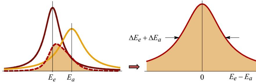
**Figure 3: Convolution of emitter and absorber Lorentzian distributions.** The left graph shows the two distributions for an assumed  $E_e$  and  $E_a$ . The shaded area is the integral of the product of the two Lorentzians. Plotting the value of this integral as a function of their energy difference results in the right graph, a Lorentzian with FWHM equal to the sum of the emitter and absorber widths.
