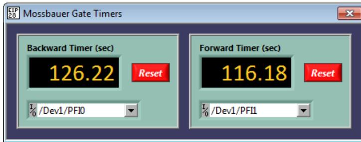
Figure 12: The Mossbauer Gate Timers application uses the mode controller gate signals connected to the computer DAQ to time the acquisitions. The times are then used to calculate the photon detection rates and the absorber velocities.
