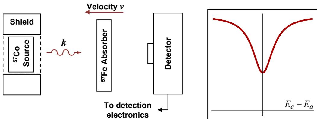
**Figure 5: Conceptual setup of the experiment. By changing the relative velocity  $v$  between the absorber and the source, emitted photons at energy  $k$  are Doppler shifted to higher or lower energy as seen by the absorber. This effectively tunes the energy difference  $E_e - E_a$ , changing the absorption rate and thus the rate that photons reach the detector (graph at right).**
