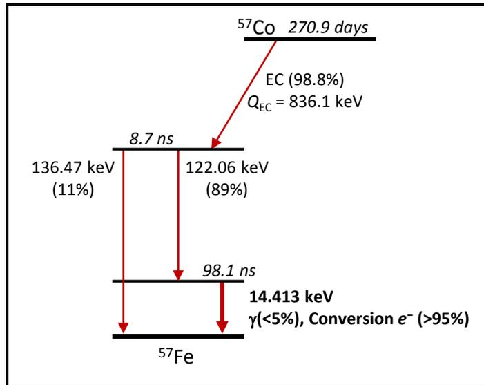
**Figure 1:**  $^{57}\text{Co}$  decay scheme showing the relevant  $^{57}\text{Fe}$  levels and emissions. The 14.413 keV transition is used for this experiment. State *half-life* times are also listed.
