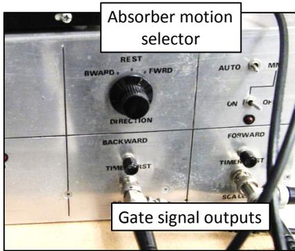
Figure 9 (left): The Mode Controller has a rotary switch which selects the direction of absorber motion: Forward (blue-shift), Backward (red-shift), or Rest (stopped). The controller then activates the motor in the proper direction. When the carriage photocell is activated, the controller sends a gate signal to activate the appropriate event counter and DAQ timer. The controller automatically stops the motor when the carriage motion limit is reached.
