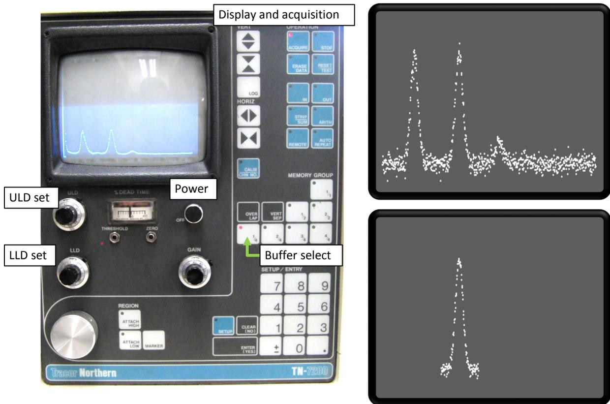
**Figure 11:** The MCA (left) must be powered on and a memory buffer selected (1/4 is a good choice). Use the display and acquisition controls to acquire photon energy spectra from the source.
