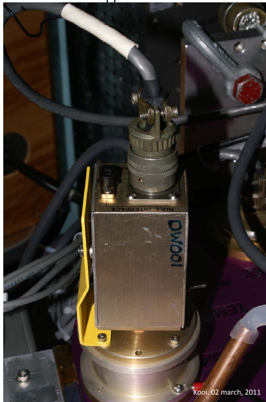
SIS Preamp change to MDM-15 with support bracket.
